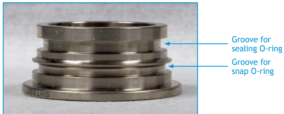
Figure 1-13: Close up of O-ring grooves in puck top
