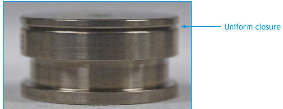
Figure 1-16: Uniform closure in properly assembled puck
