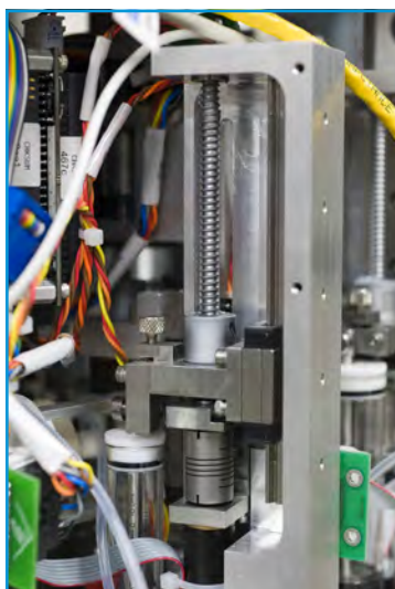
Figure 1-6: Syringe ballscrew assembly
