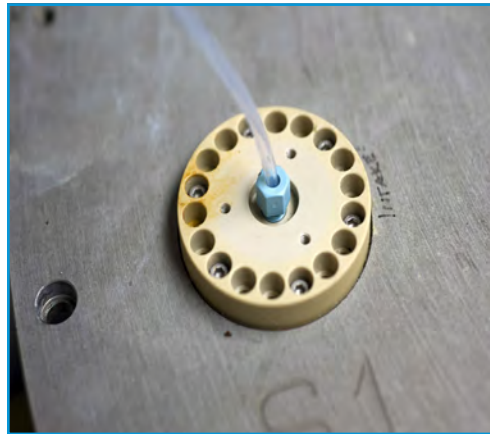
Figure 1-14: Sampling tube connected to Intake Port
