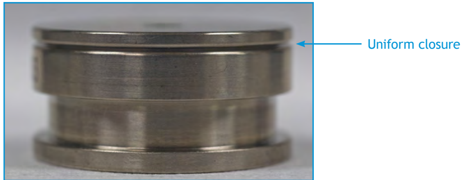
Figure 1-14: Uniform closure in properly assembled puck
