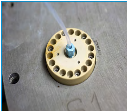
Figure 1-9: Supply line connected to Intake Port
